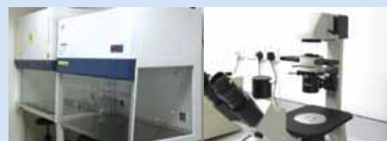
Tissue-culture facility which houses laminar air flow hood, biohazard laminar flow and inverted microscope
